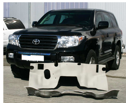
Deform hot forms and quenches and tempers armour plate. This is a fire-wall for the Toyota LC200.
